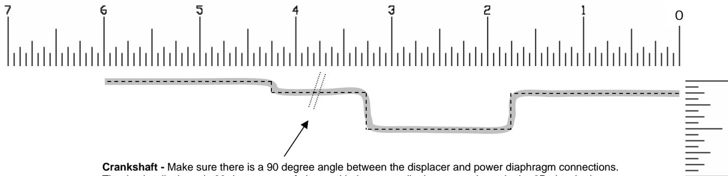
**Crankshaft** - Make sure there is a 90 degree angle between the displacer and power diaphragm connections. That is, the displacer is 90 degrees out of phase with the power diaphragm as shown in the 3D sketch above. Use 7 inches of coat hanger wire (or equivalent) to make the crankshaft.
